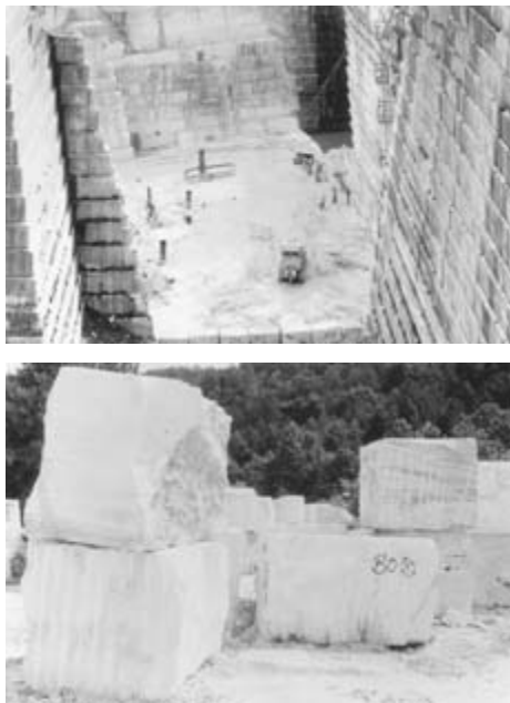
Figure 5-2 Quarrying stone. (Photo courtesy Georgia Marble Co.)
