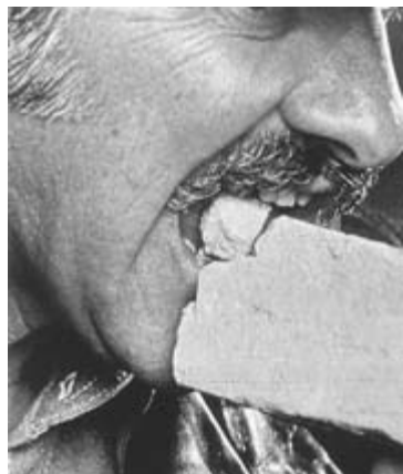
Figure 3-4 Substandard brick. (Photos courtesy Brick Institute of Texas.)
