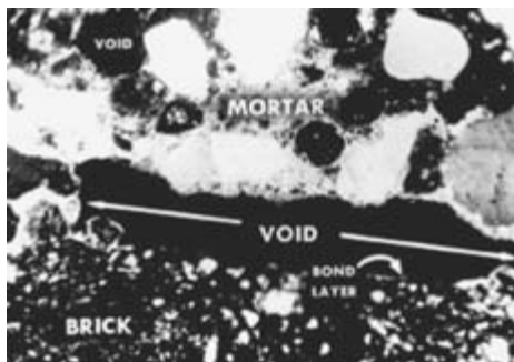
Figure 6-5 Microscopic view of mortar bond line. (Photos courtesy National Lime Association.)
